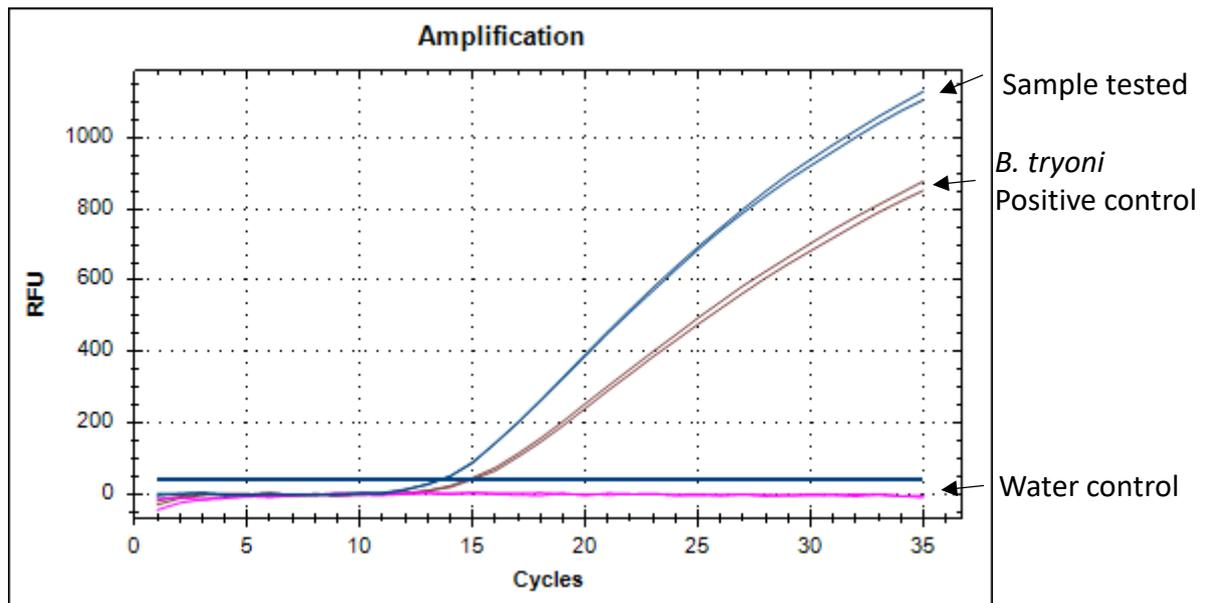
Amplification curves of real-time PCR assay for *B. tryoni* complex. The sample tested positive for *B. tryoni* complex, DNA sequences has further confirmed the results.
